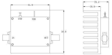
Including a small heatsink without Fan if output Power higher than +20dBm.
