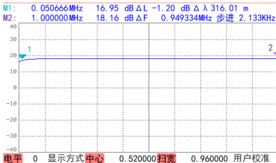
Gain vs Frequency 50kHz-1MHz
